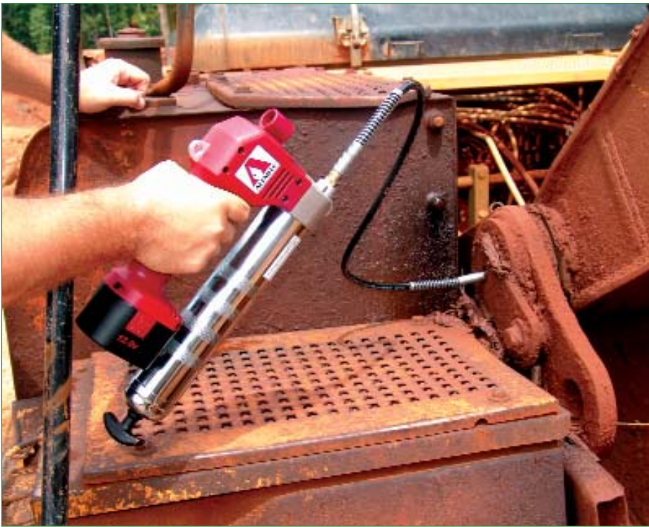
An Alemite battery operated grease gun is used to lubricate bearings. Grease guns are still the best option for lubrication in some situations. Battery operated grease guns make manual lubrication quicker and more efficient than manual grease guns.
