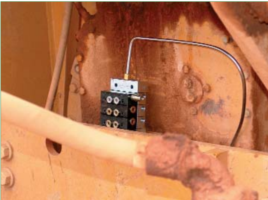
An Alemite high pressure series modular divider valve is used to supply lubricant to points on off-road equipment.
