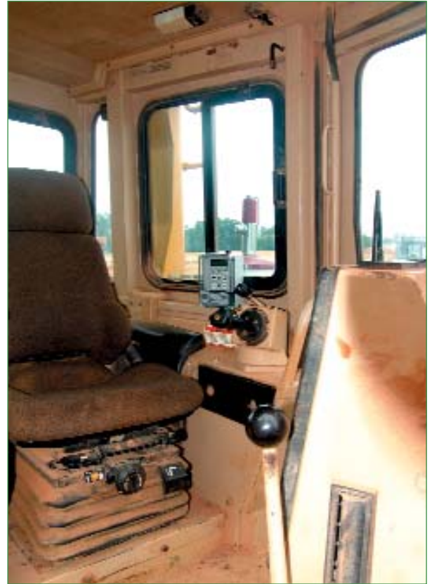
The Alemite CLS 1000 controller is used to activate a pump that supplies the injectors with lubricant. The controller allows remote monitoring and control of automatic lubrication equipment.
